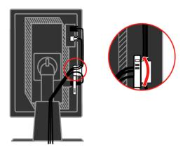
Wrap the Cable Wapper around the cables. 7.
